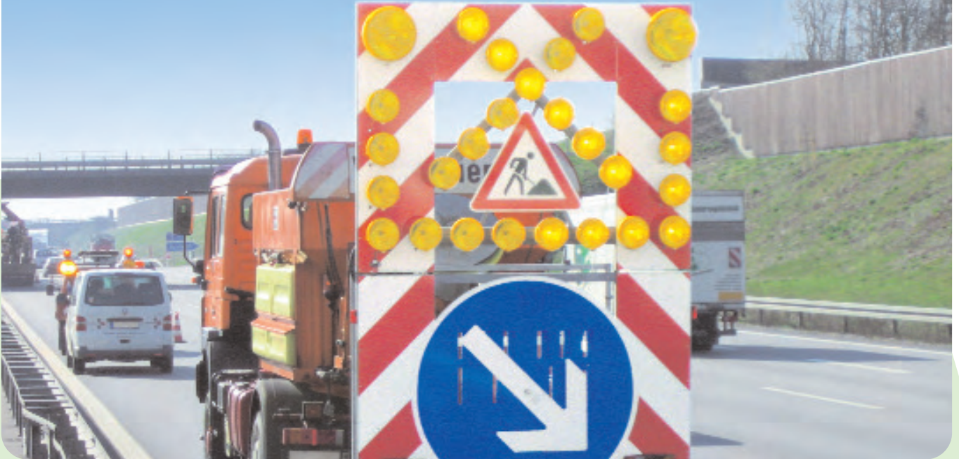
Traffic guidance system of Autobahnmeisterei München-Nord
