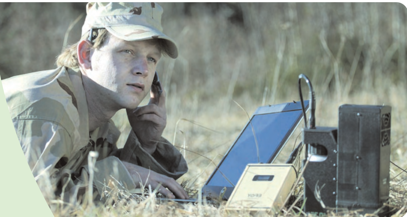
Jenny-Fuel Cell and Power Manager – portable power supply in the field
